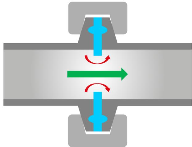
Figure 6 - Over compressed gasket protruding into pipework
