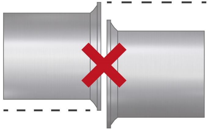
Figure 3 - Ferrules must be completely aligned
