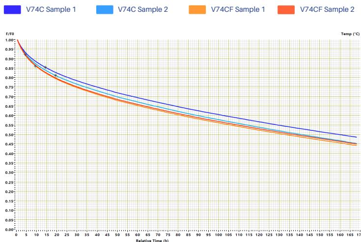
High temperature performance has been compared using compressive stress relaxation ISO 3384-1 Method B at a constant temperature of 240°C (464°F) for 168 hours with -214 O-Rings under 25% compression.
