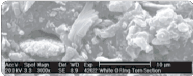
Figure 1: Inorganic filled elastomer material (magnification 10µm)
