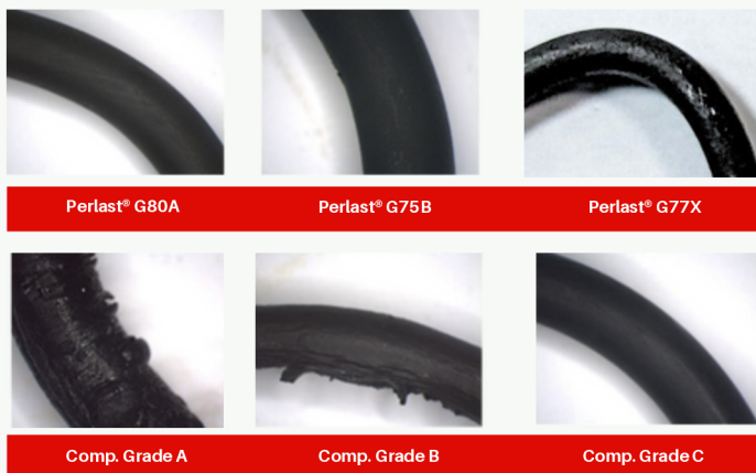
Images of the O-ring surfaces after ageing 20 x magnification
