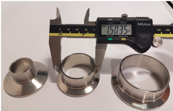
Figure 2 - Measuring the outside diameter of the tube on a 1½" ferrule
