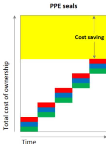
Here we can clearly see the impact of two premature failures of the low cost seal, compared to the PPE seals, over the same period of time. The increased installation cost and extended downtime results in much higher cost of ownership. Seals that provide consistent reliable service life allow preventative maintenance to be carried out on schedule.
