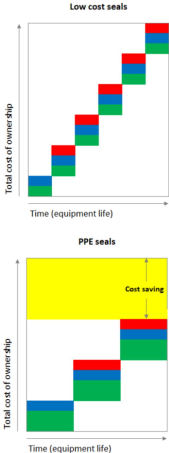
In this instance, the low cost seals work out more expensive in the long-term. Typical scenarios where this might occur are buying cheap imports from the Far East or using lower spec' materials such as EPDM. By swapping them out for high quality seals or upgrading the material to a higher performance material (such as FKM), seal life is increased and overall cost savings can be achieved.
