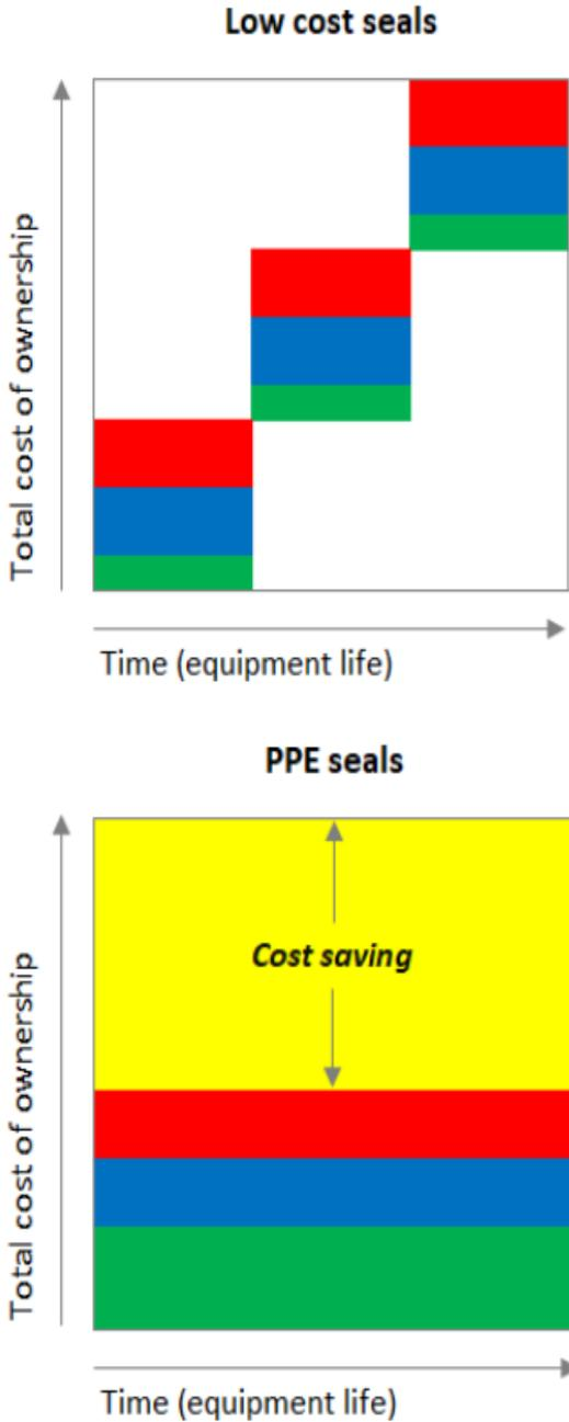
Here, the PPE seal acquisition cost is x3 compared to the low-cost seal option. However, the PPE seal lasts x3 longer, so its total cost of ownership is half that of the low-cost seal that needs changing twice, due to its reduced service life. An overall cost saving is achieved by extending the maintenance intervals and eliminating the additional installation and downtime costs.
