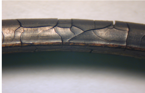
Example of thermal embrittlement of seal
